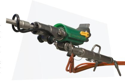
The ST 185 also has an improved rubber grip handle that dampens vibrations; and a hand guard that protects the RDO from crushing his hand in the event of an air leg rise, which is a common problem underground.
